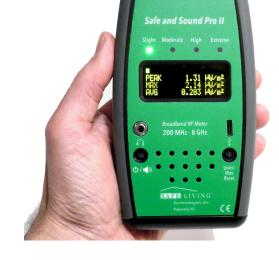
This sensitive meter is capable of measuring potentially harmful RF or microwave radiation from any continuous or pulsed digital sources. To help identify these various sources, the Safe and Sound Pro II includes a built in speaker with adjustable volume levels. Each source has its own unique sound signature.
