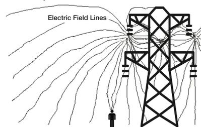
AC Electric Fields: jagged field lines lines from a radiant source, which travel to places of lower electrical potential or to ground.
