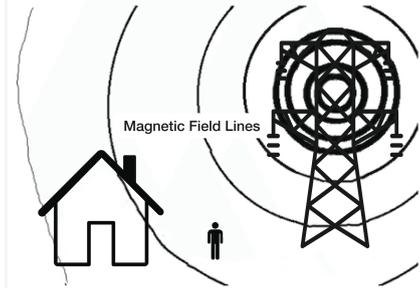
AC Magnetic Fields: concentric rings radiating from a source, which decrease with distance.
